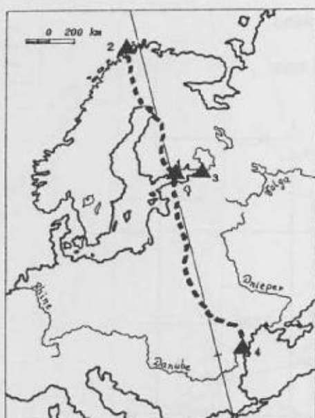
- - - - - RSAM triangulation row + - - - - arc of the meridian ▲ stations of the 1994 GPS experiment: 1 - MÄKIPÄÄLLYS 2 - FUGLENESET 3 - PULKOVO 4 - STARAJA NĚKRASOVKA
